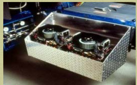
PEM FC Integrated by Xcellsis into the Prototype
