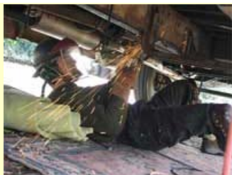
Chris Congleton welds under his LPG conversion bus project
