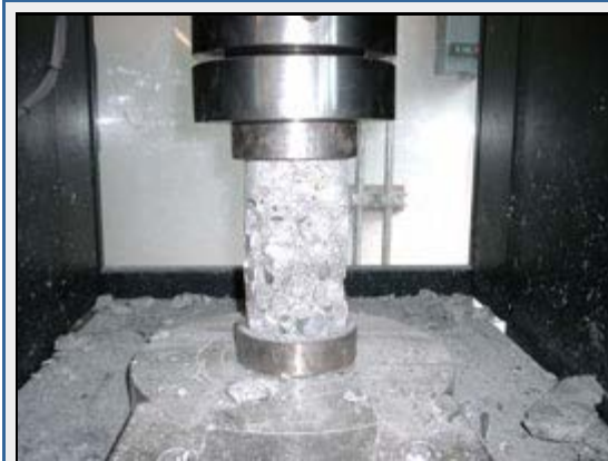
A four-inch diameter concrete core after compression testing. Data from the test will be used for a research project involving mechanistic-empirical pavement calculation methods.
